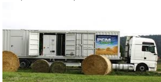
Photo 2: PCM Green Energy; mobile pelleting line - "MBA 1000" [47].
