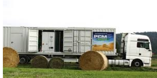
Photo 2: PCM Green Energy; mobile pelleting line - "MBA 1000" [47].
